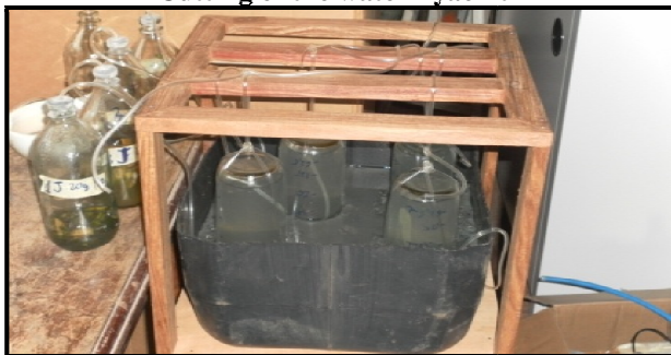
Figure-2 Experimental setup of the BMP test
