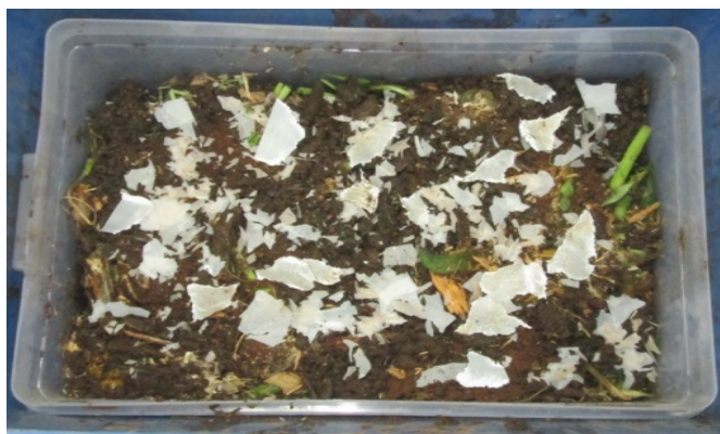
Figure-2: Addition of plastic sheet sample.
