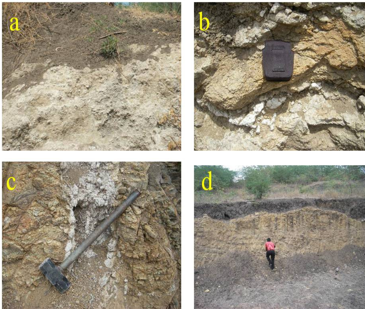
Figure-2(a-d): a-The field photographs show a surfacial outcrop of black soil and thick calcrete profile deposits in the river section. b-The field photographs show the chalky deposits within fracture zone of exposed weathered sap rock. c-The field photograph shows the calcrete deposits as discordant form in the exposed weathered sap rock. d-The field photographs show the bottom weathered sap rock of granite and charnockite followed by calcrete profile and top black soil.
