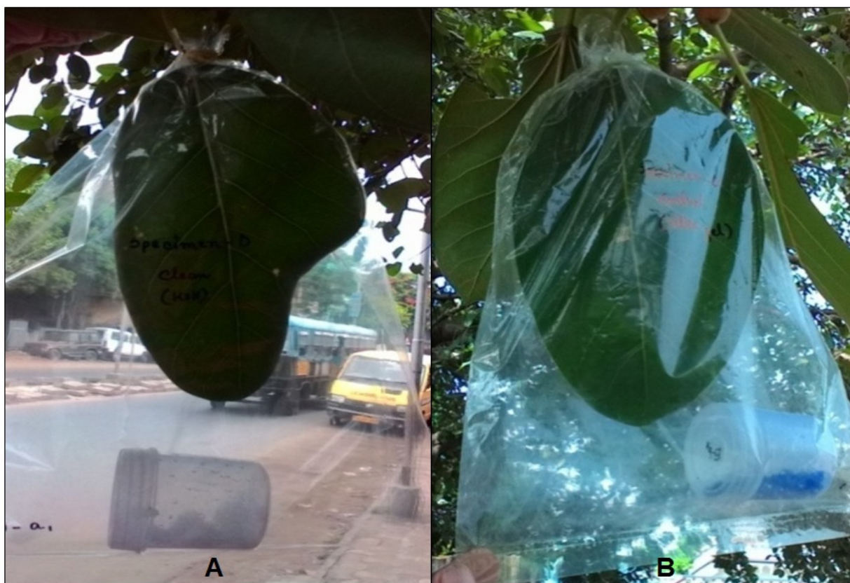
Figure-1: Experimental setup to measure reduction in O 2 release due to dust deposition (A- with silica gel crystals, B- with KOH pellets)
