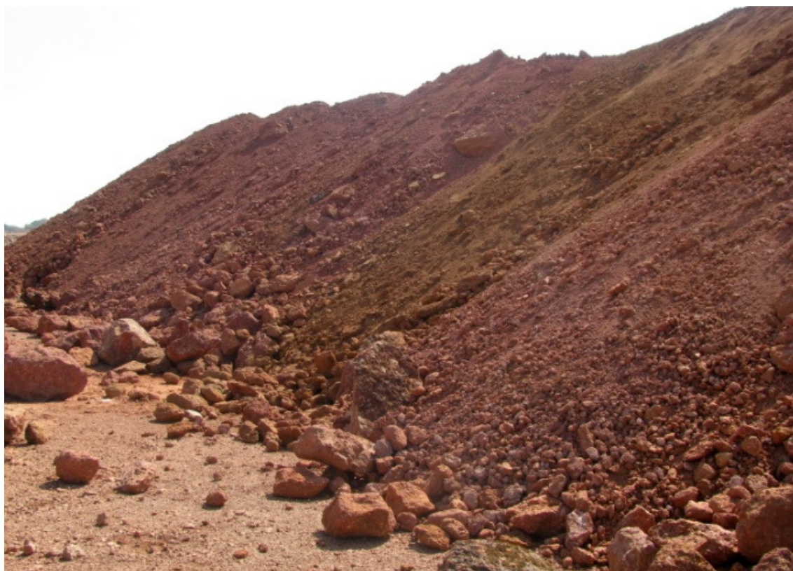
Figure-3 Overburden dump without retaining walls M/S Swati Minerals, Udgiri
