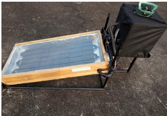
Figure-8: Flat plate solar collector realised.
