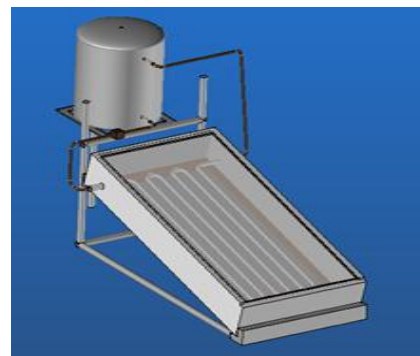
Figure-6: Flat plate solar heat collector.
