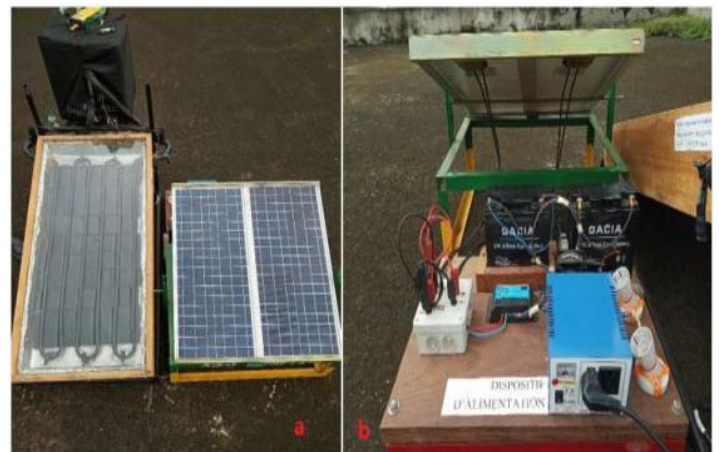
Figure-10: (a) Flat plate thermal collector + Photovoltaic solar panels; (b) Solar power device (DC/AC).
