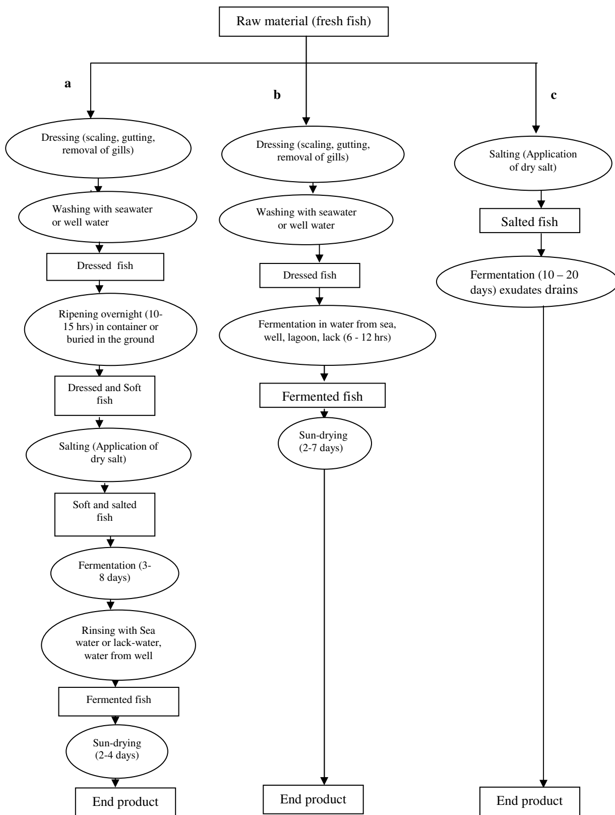
Figure-1 Flow diagram of traditional processing of fermented fish products in Africa
