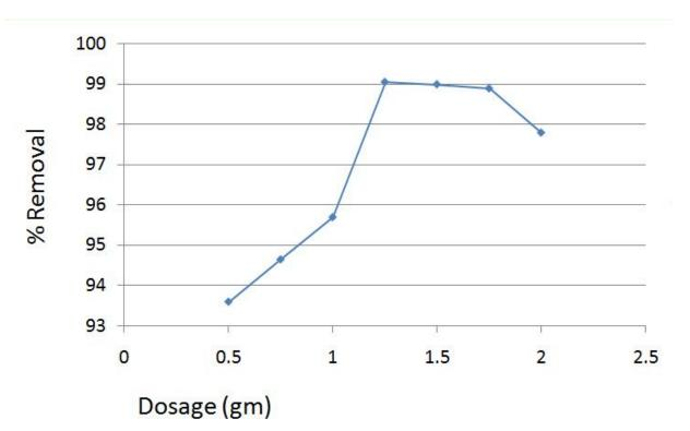
Figure-2 Effect of dosage on the adsorption of Ni by Maize cob
