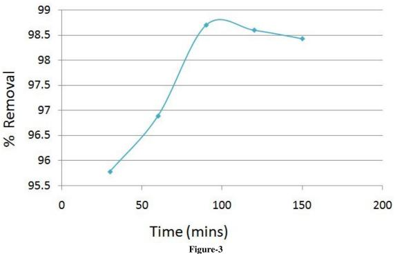
Figure-3 Effect of time on the adsorption of Ni by Maize cob
