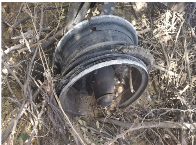
Figure-5: A view of completely burnt right rear tire.
