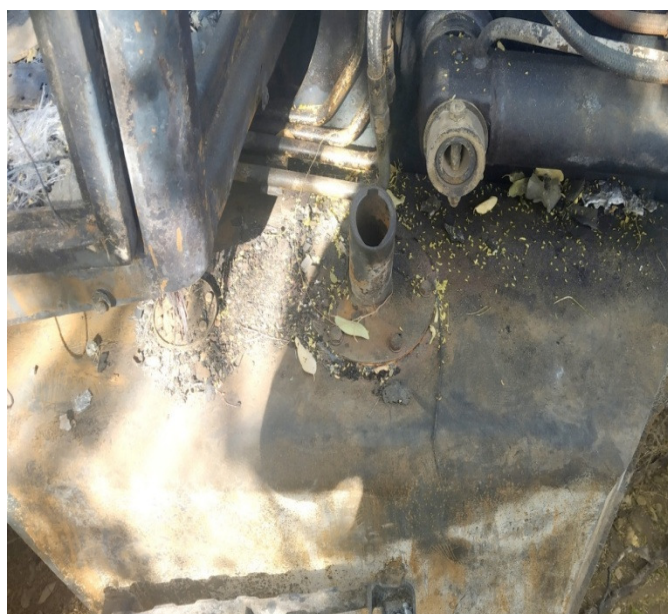
Figure-7: Diesel tank unaffected by fire.
