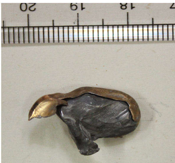
Figure-2: Photographic match fit of lead core and copper jacket.
