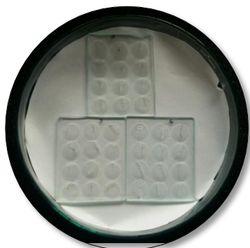
Figure-3: Each thread attached to the cavity slide with dpx mount.
