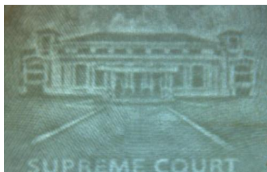
Figure-2: Watermark (Supreme Court) in the paper substrate of passport of Republic of Ghana.
