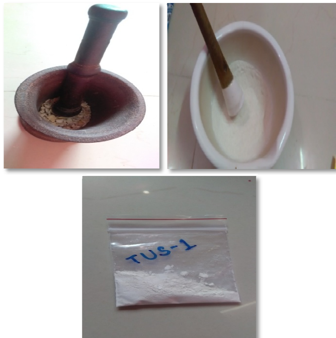
Figure-2: Crushing of samples using iron mortar and agate mortar and pestle.
