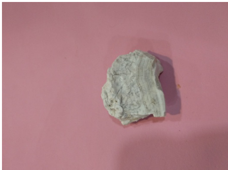
Figure-9: Full formed silica rock (white) from basaltic Rock found at Lonar Crater Lake.
