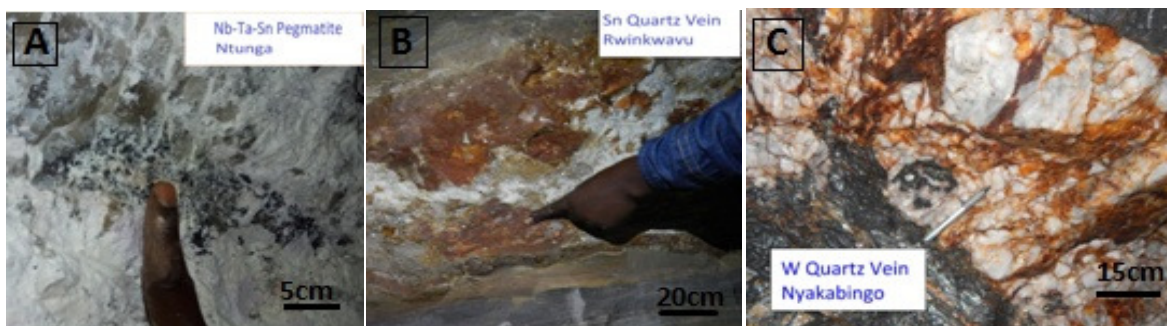
Figure-5: Field photographs taken during the field investigation. A. Intrusion of advanced argillic alteration of pegmatites with concentrates of coltan at Ntunga. B. Quartz vein mineralized in cassiterite and hosted in schist at Rwinkwavu. C. Quartz vein mineralized in tungsten and hosted in black shale at Nyakabingo.
