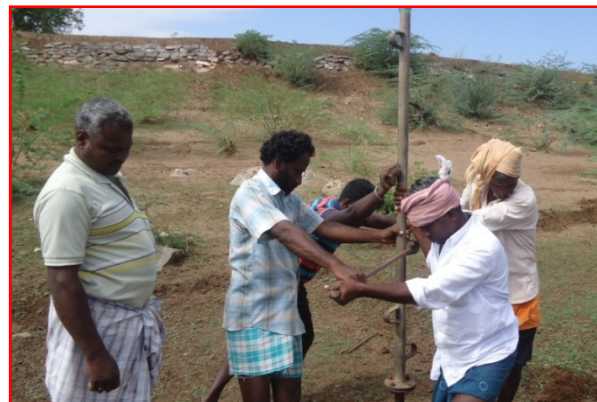
Figure-1 Sampling in Lake by Rotatory Drill
